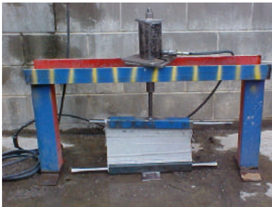
Fig 6 - In house testing of fixing system and Fabric D
