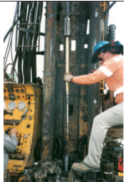
Fig 2b - Stress measurement tool about to be lowered into HQ drill rods.
