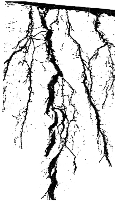
Fig. 2 - A polished and etched metallographic cross section showing typical transgranular SCC in stainless steel
